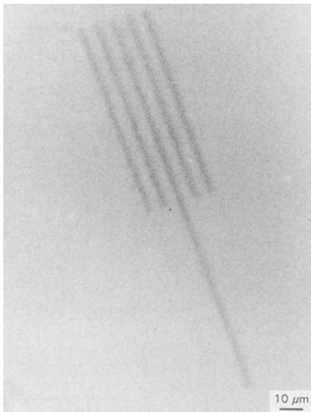
Figure 2 Scanning electron micrograph of a surface obtained by the photolithography of (dppe)Pt(Me)(N_3) on a silicon (111) surface (image obtained at a 45^\circ angle).
